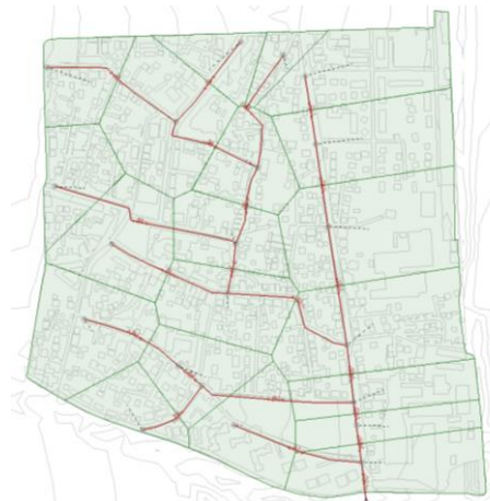
Hydraulic model - storm sewerage network
