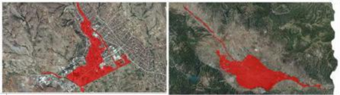
Figure 17 –Potential Q_{100} floods in Radovish city (by torrents Sushica, Radovishka Reka) and Radovish-Strumica valley (by river Strumica)
