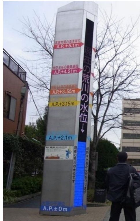
Water level is displayed in real time water levels of past flood are shown
